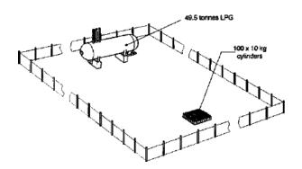
The separation between the compound and the large tank is sufficient to prevent the cylinders starting a major incident at the large tank.
