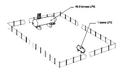
The small tank = 2% of medium hazard threshold (50 tonnes), but the separation from the large tank is sufficient to prevent the small tank starting a major incident at the large tank. It can therefore be ignored in terms of the 2% rule.
