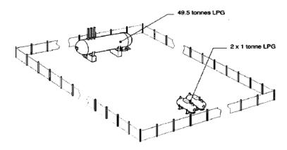
The small tanks are adjacent to each other but their separation from the large tank is not sufficient to prevent the small tanks starting a major incident at the large tank.
