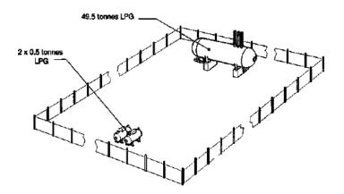
The small tanks are adjacent to each other but well separated from the large tank.
